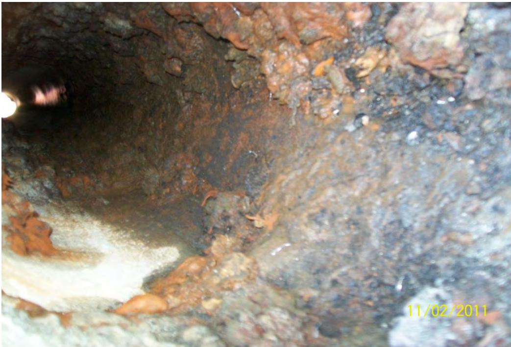
Photo 16 : Inside of water main pipe removed for repair.
