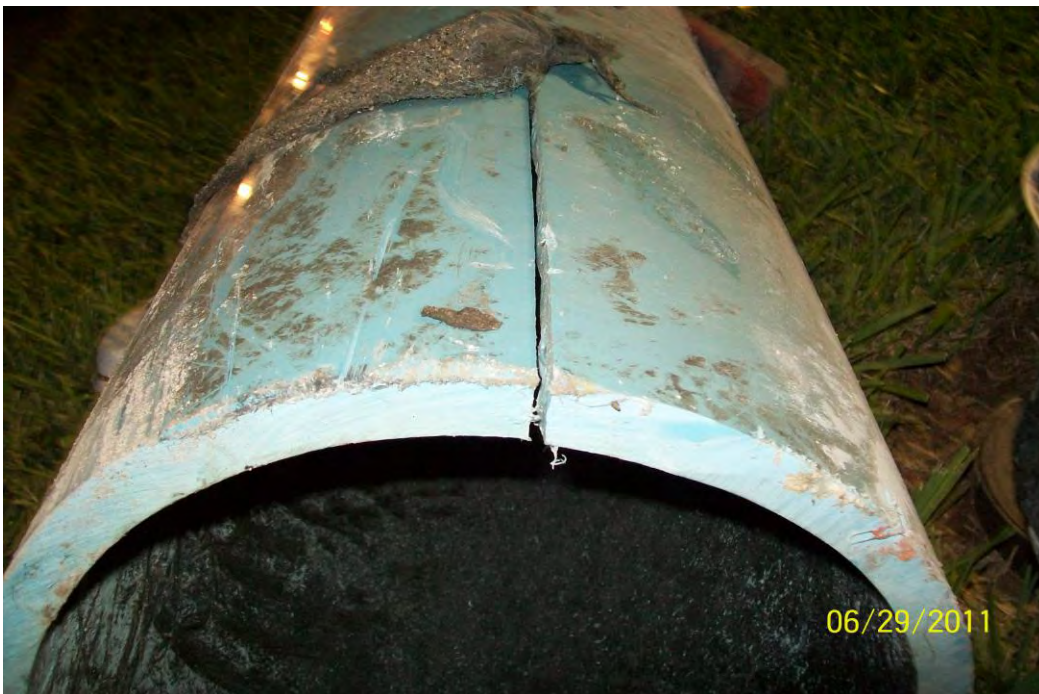
Photo 8: Longitudinal crack of PVC Sanitary Force Main.
