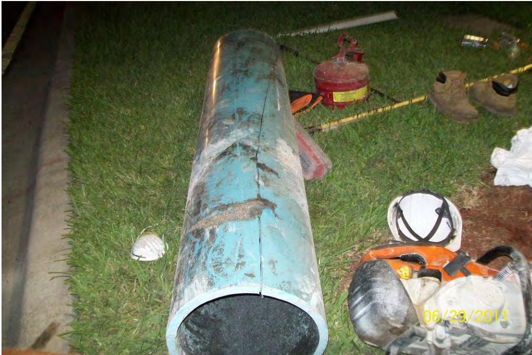
Photo 7: Longitudinal crack of PVC Sanitary Force Main.
