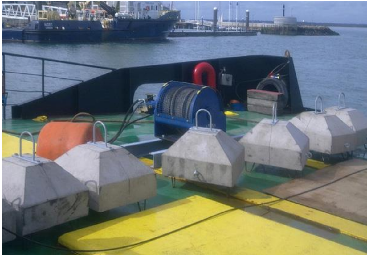
Concrete block anchors
