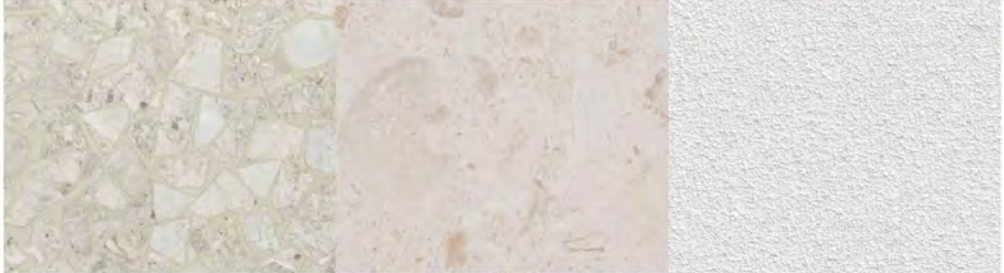
1 PROPOSED STONE WALL CLADDING 2 PROPOSED PAVERS ON POOL DECK, IVORY SHELL STONE 3 PAINTED SMOOTH STUCCO FINISH, COLOR TO MATCH EXISTING BLDG
